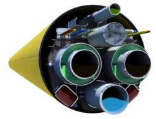
Cross Section of a Pipeline Bundle
